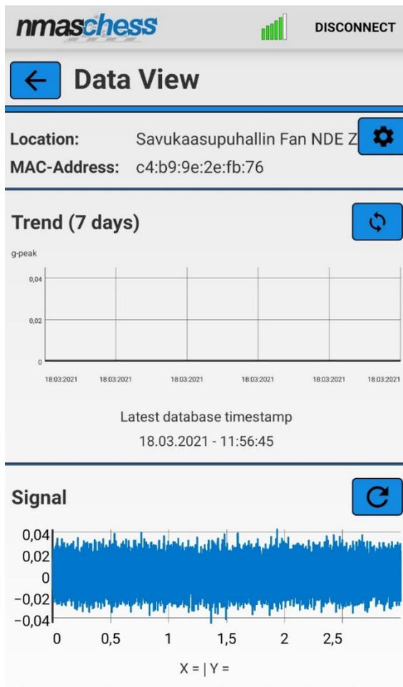
The values shown on the trend are gpeak and the trend updates automatically as new measurements are done. The trend can also be updated manually with the button on the right side of the screen. Below the trend is latest database timestamp which shows the time of the last measurement that has been transferred to database. If there are warning- and alarm-limits set for this location, those will be shown on the trend.
